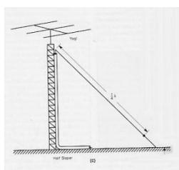
Another antenna that is being used successfully at VE9ML is the sloper. Since I have a 65ft tower, it was decided to put up three 80m  $\frac{1}{4}$  wave slopers in various directions. They do give a small bit of directivity, but the sloper is basically a vertical antenna with an omni directional radiation pattern. This is a very easy way to improve your 80m signal/reception. Vertical antennas work very well on the lower bands since they have a low take off angle.
